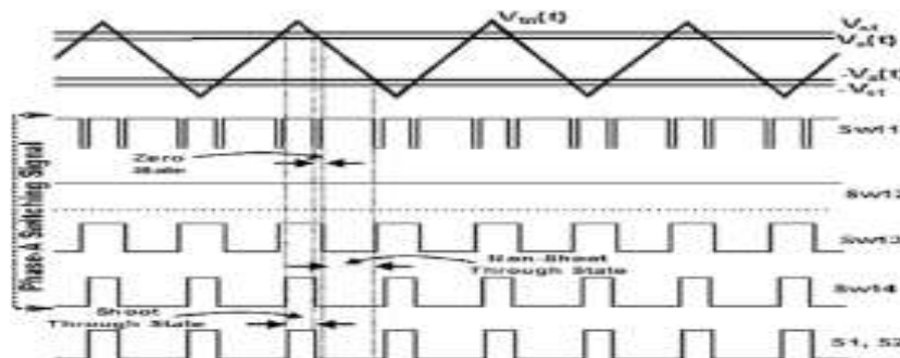
Fig.5.PWM control of LC-Switching voltage boost NPC inverter
